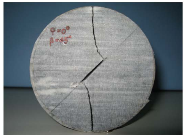
Figure 17 Photograph of specimen AM-4 after failure ( \psi = 0^\circ and \beta = 45^\circ ).
