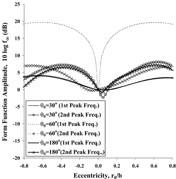
Fig. 4. The form function amplitude versus the source eccentricity at the first and second peak frequencies for the radially vibrating piston at selected cap angles.
