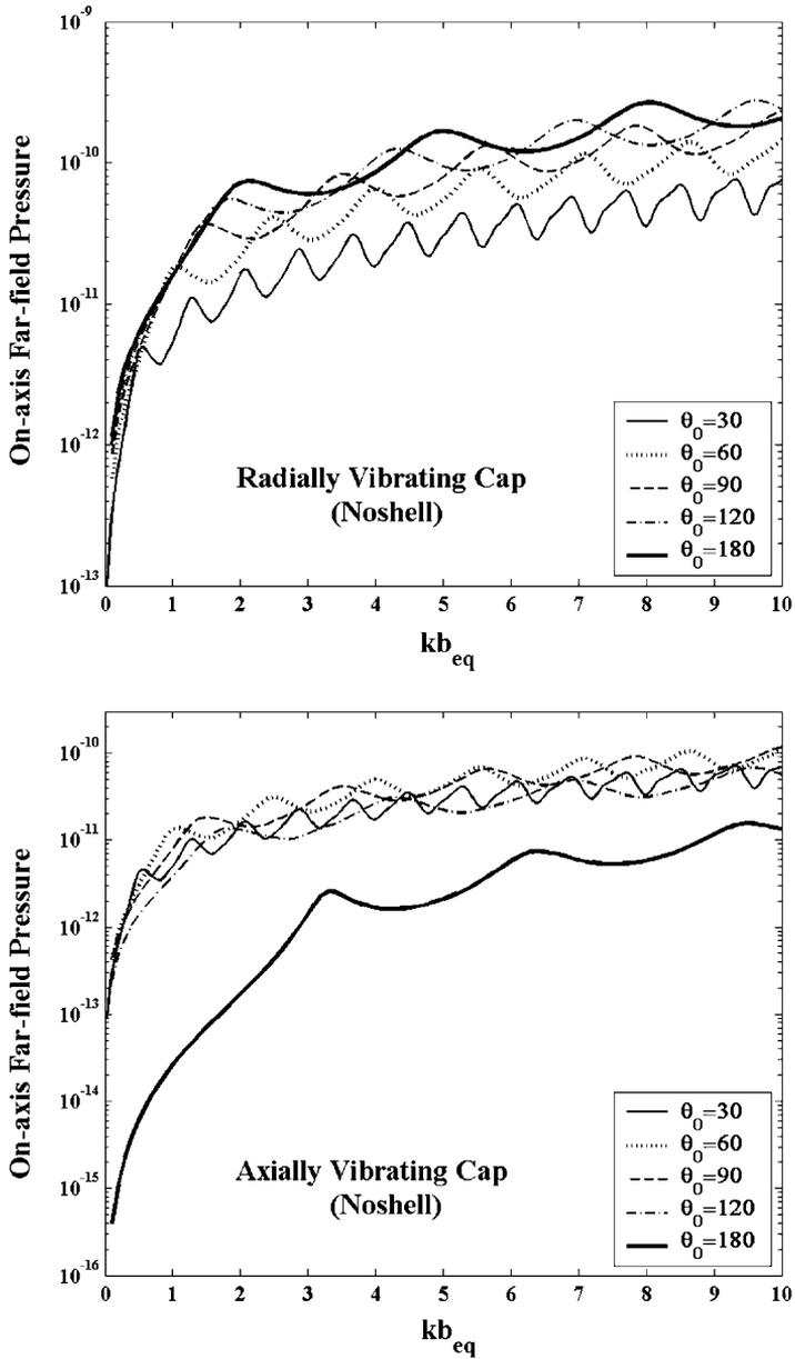
Fig. 3. The change in the on-axis far-field pressure magnitude with the nondimensional frequency for the radially/axially vibrating piston positioned in the center of the fluid sphere for selected the cap angles.
