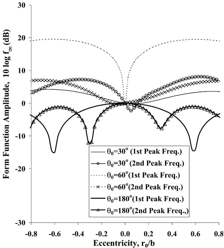
Fig. 5. The form function amplitude versus the source eccentricity at the first and second peak frequencies for the axially vibrating piston at selected cap angles.
