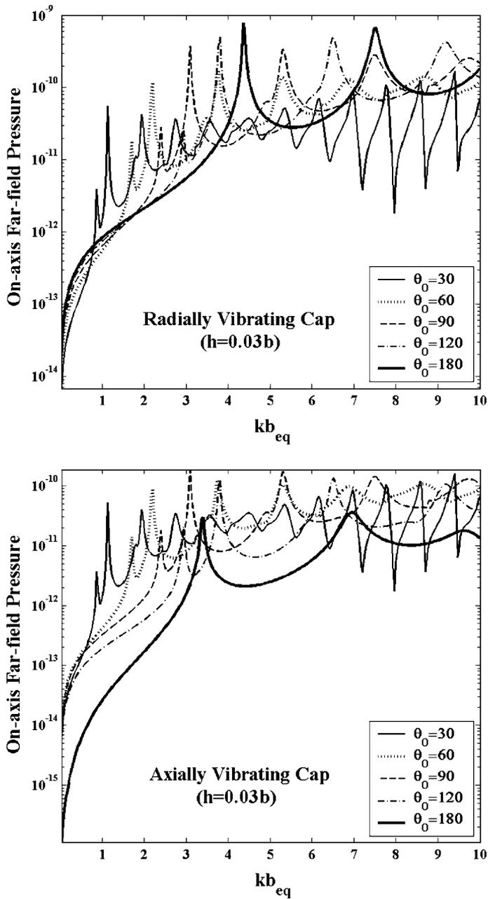
Fig. 2. The change in the on-axis far-field pressure magnitude with the nondimensional frequency for the radially/axially vibrating piston positioned in the center of the elastic shell for selected the cap angles.
