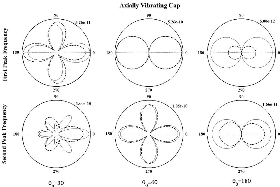
Fig. 7. The influence of cap angle on angular distribution of the radiated far-field pressure at the primary and secondary focal points corresponding to the first and second peak frequencies of the shell-encapsulated axially vibrating piston (the solid/dashed line curves correspond to the primary/secondary focal points).
