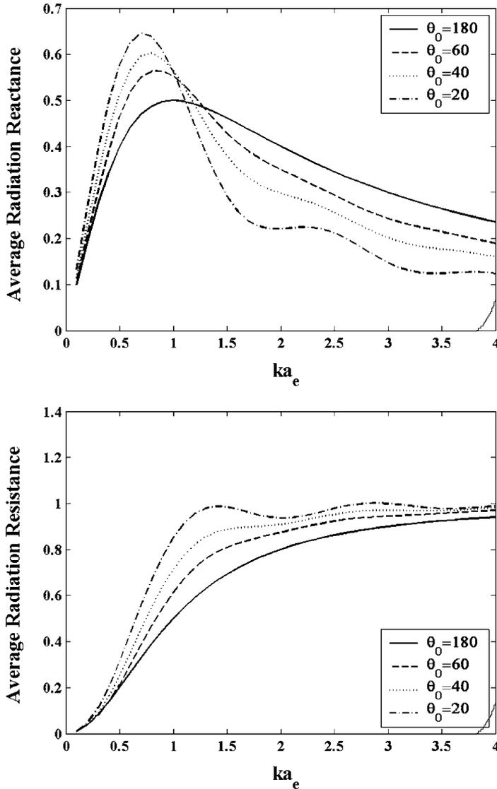
Fig. 8. Acoustic radiation impedance components for a baffled pulsating spherical cap, suspended inside a water-filled (very) light and thin spherical shell immersed in water, as a function of  $kb_e$  ( $h \approx 0.0001b$ ,  $\rho_s = \rho = \rho^* \approx 1 \text{ g/cm}^3$ ).
