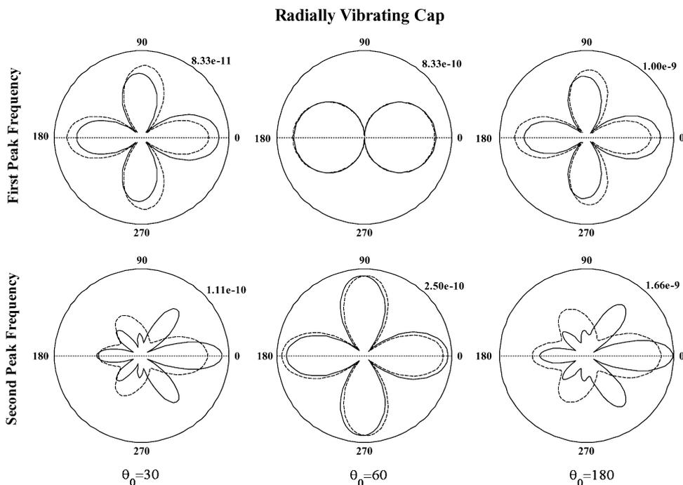
Fig. 6. The influence of cap angle on angular distribution of the radiated far-field pressure at the primary and secondary focal points corresponding to the first and second peak frequencies of the shell-encapsulated radially vibrating piston (the solid/dashed line curves correspond to the primary/secondary focal points).
