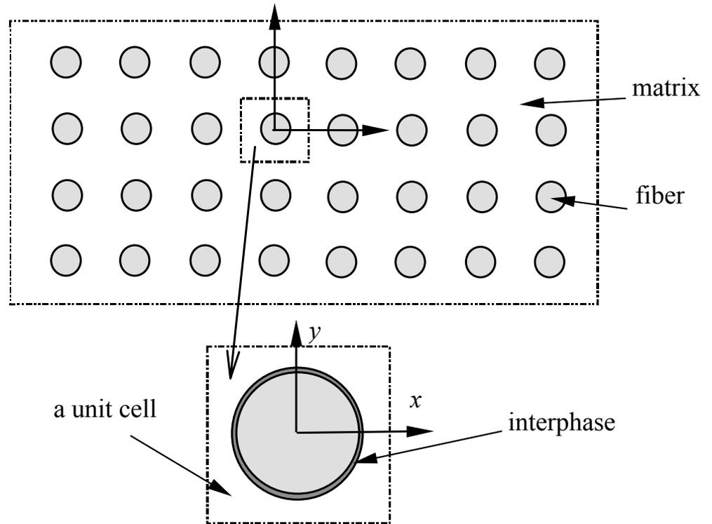
Interphases in fiber-reinforced composites are modeled using the BEM and FEM to investigate their effects on the mechanical properties and interface failures of the material.
