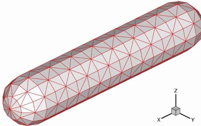
A BEM mesh used for the short fiber inclusion (with 456 constant elements)
