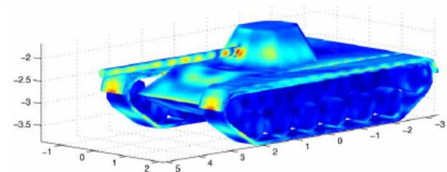
Electromagnetic wave scatterings from targets
