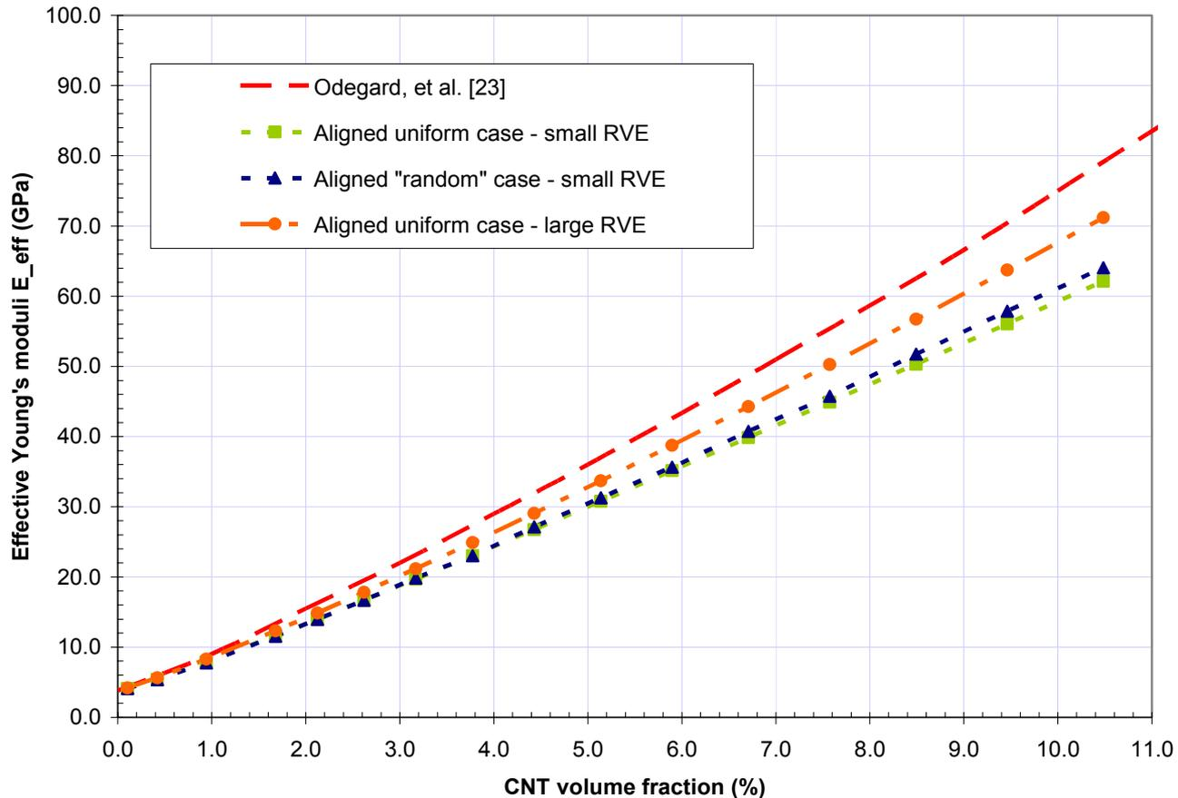
Computed effective moduli of CNT/polymer composites using three RVEs and compared with NASA's multi-scale results
