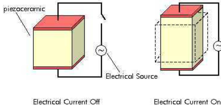
The mechanical and electrical coupling effect in piezoelectric materials
