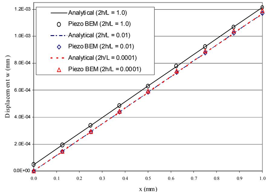
Displacement component  $w$  along the bottom edge of the strip ( $M = 24$ ) for different thicknesses
