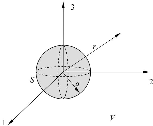
A sphere with tri-axial loading
