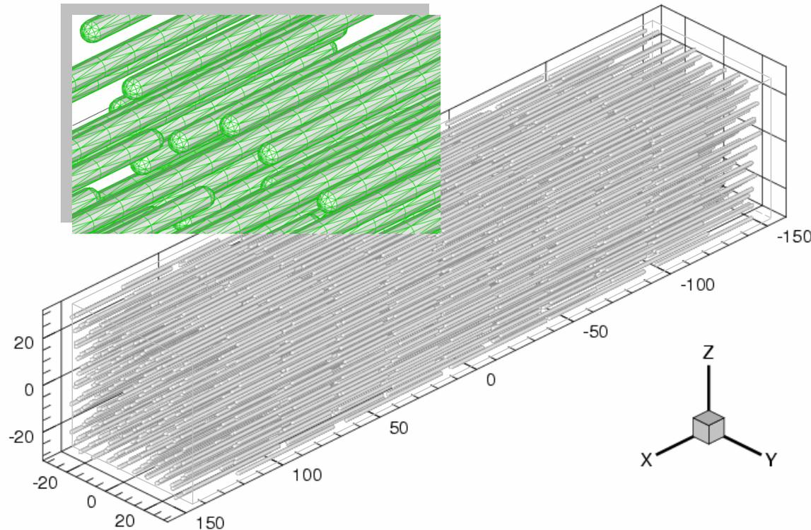
A small RVE containing 2,000 CNT fibers with the total DOF = 3,612,000 (CNT length = 50 nm, volume fraction = 10.48%). A larger model with **16,000 CNT fibers** and **28.9M DOFs** was solved successfully on a FUJITSU HPC2500 supercomputer (at the Kyoto University) within 34 hours.
