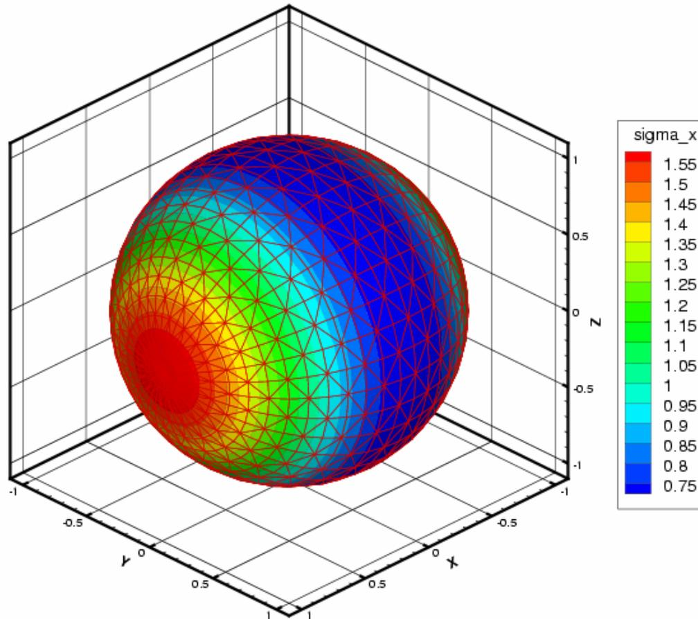
Contour plot for stress on the surface of the sphere
