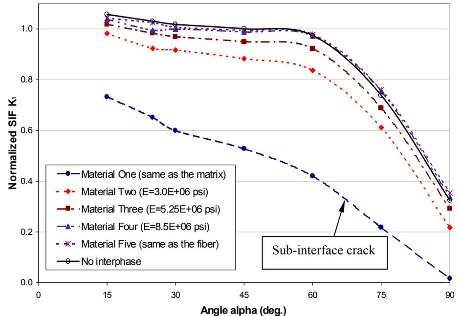
Effects of the interphase materials on the stress intensity factor ( $K_1 / \sigma_{ave} \sqrt{\pi R \alpha}$ ) for the circular-arc interface crack
