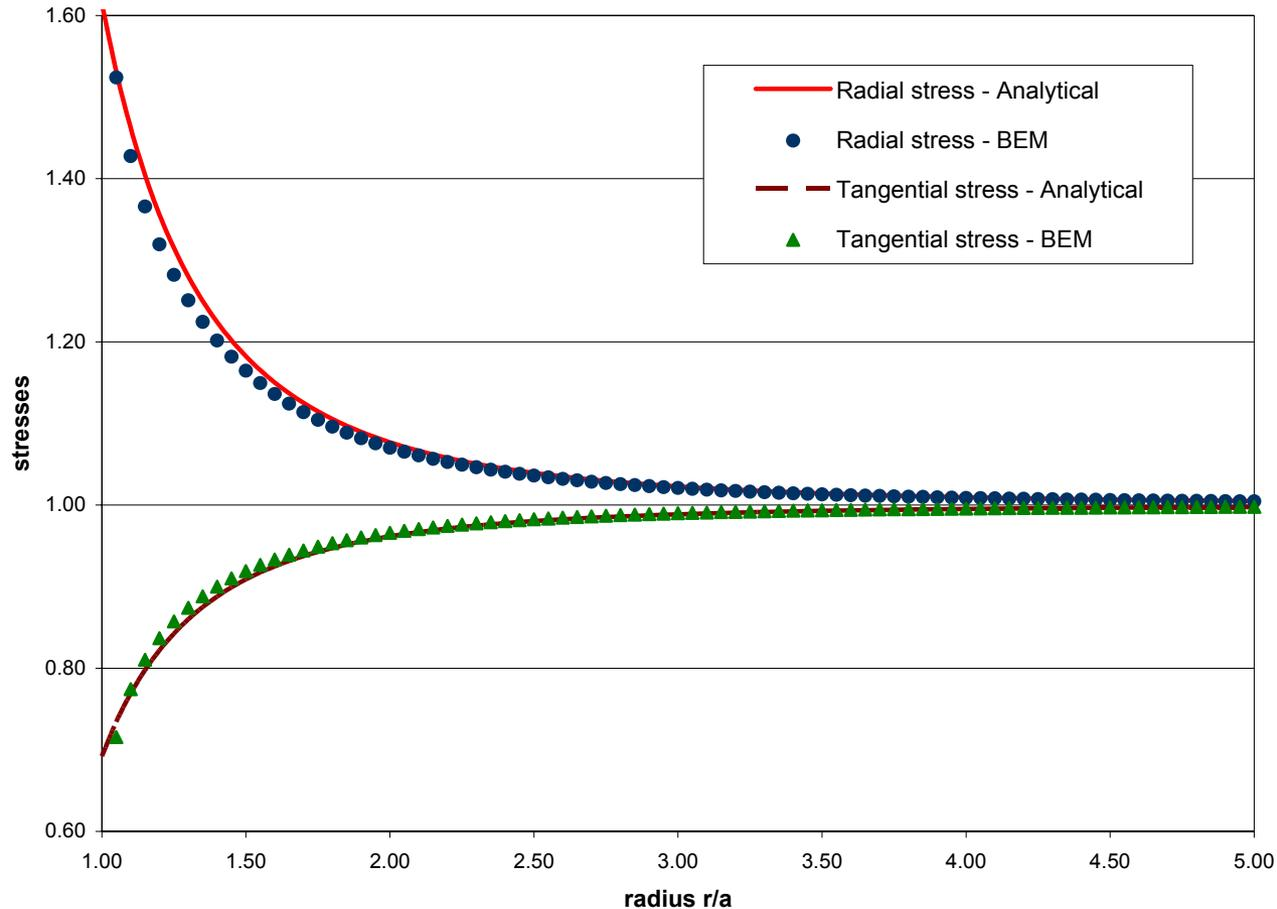
Radial and tangential stresses obtained by a BEM model with 120 elements
