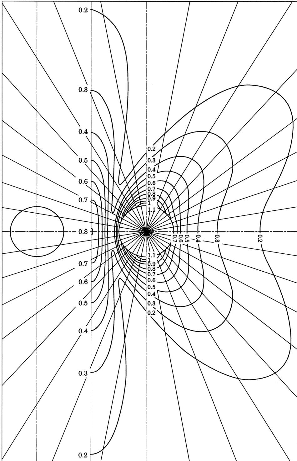
Figure 6. Equal pressure contours of two dilating spherical sources at the  $z=0$  plane for  $ka=2$ .
