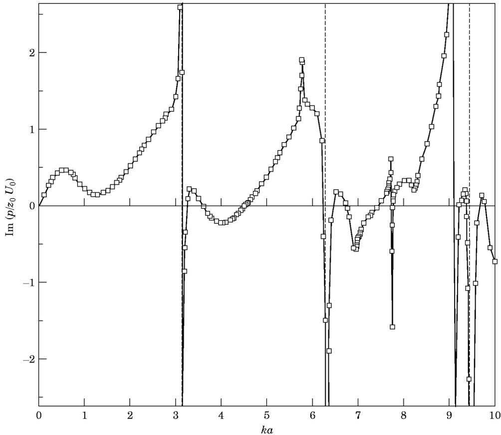
Figure 9. Variation of the imaginary part of the non-dimensional surface pressure at the nearest points of the equatorial circles of two dilating spherical sources, computed by using SHIE, with the non-dimensional wavenumber  $ka$ .
