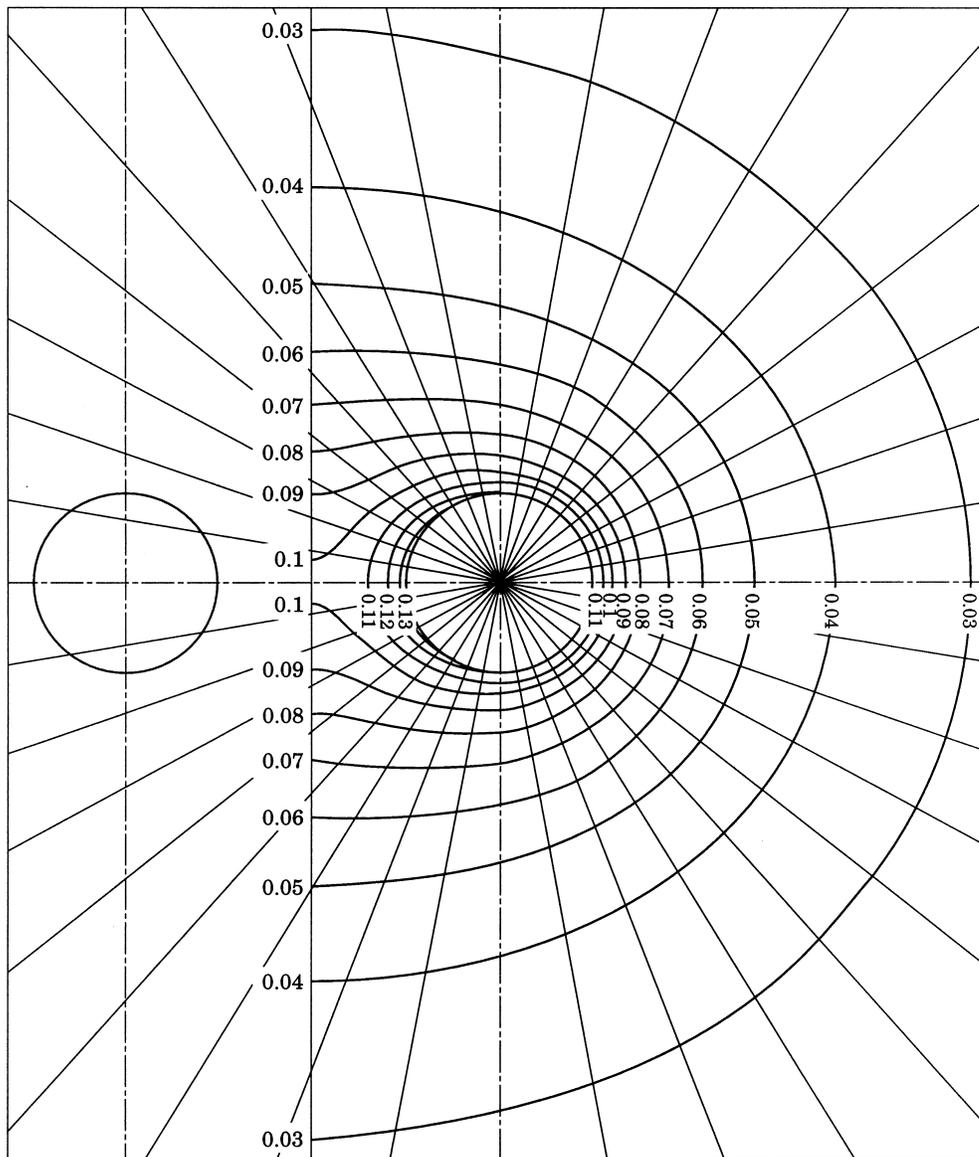
Figure 5. Equal pressure contours of two dilating spherical sources at the  $z=0$  plane for  $ka=0.1$ .
