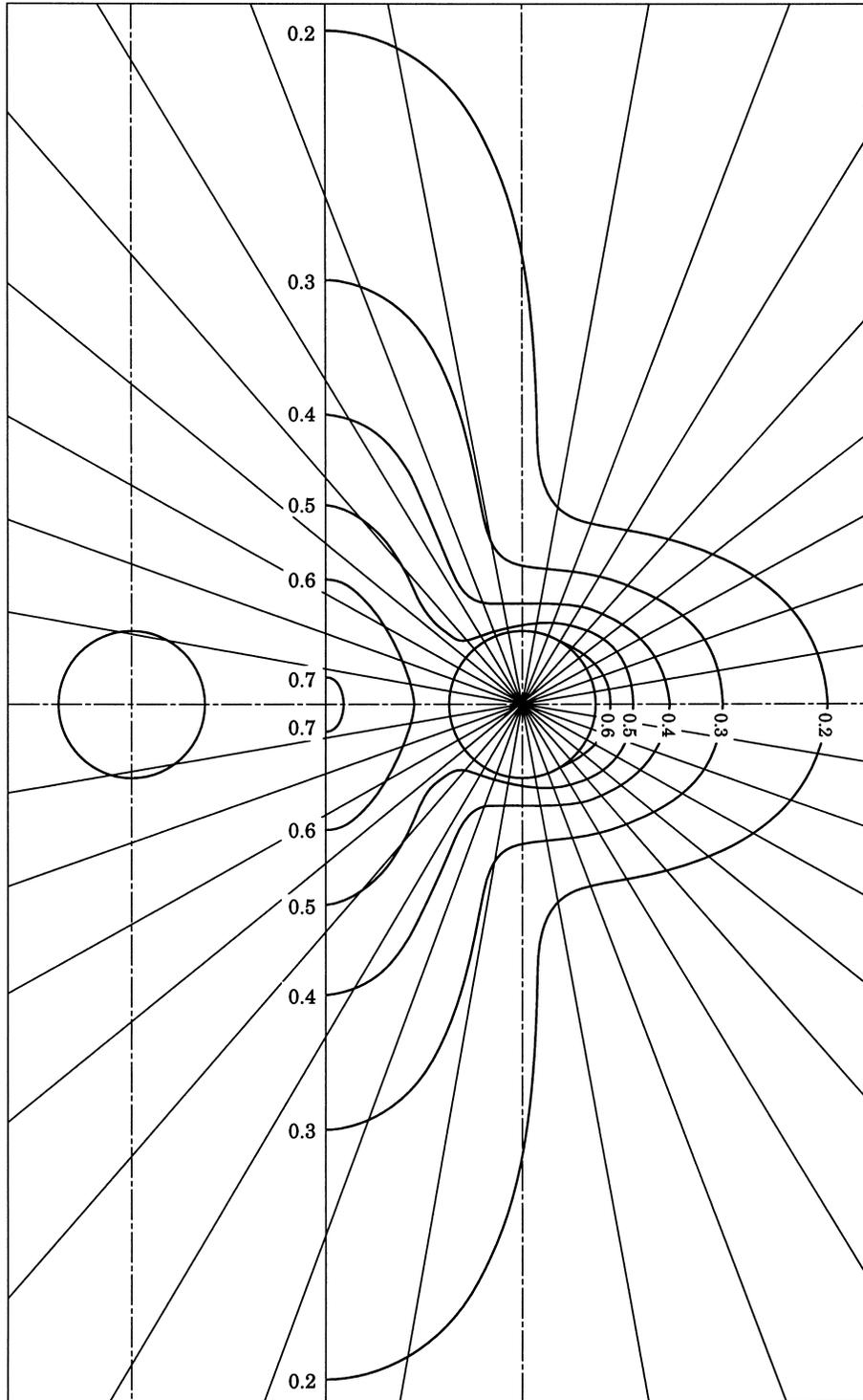
Figure 4. Equal pressure contours of two dilating spherical sources at the  $z = 2a/3$  plane for  $ka = 1$ .
