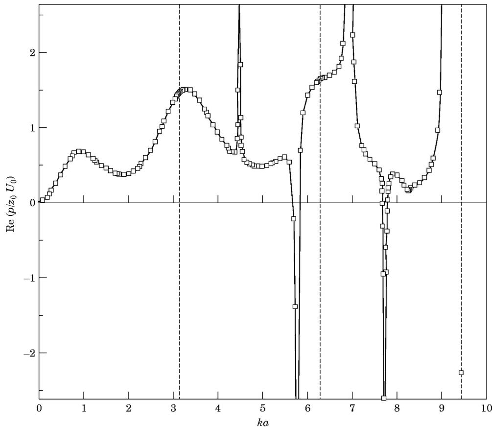
Figure 8. Variation of the real part of the non-dimensional surface pressure at the nearest points of the equatorial circles of two dilating spherical sources, computed by using CHIEF, with the non-dimensional wavenumber  $ka$ .
