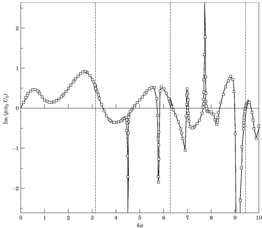
Figure 10. Variation of the imaginary part of the non-dimensional surface pressure at the nearest points of the equatorial circles of two dilating spherical sources, computed by using CHIEF, with the non-dimensional wavenumber  $ka$ .
