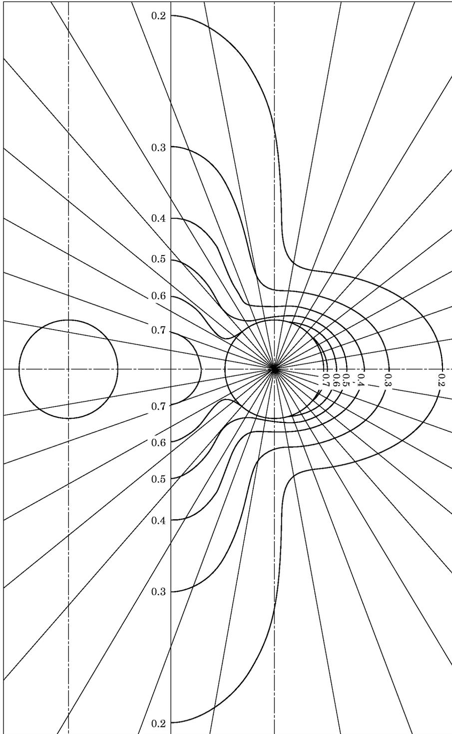
Figure 2. Equal pressure contours of two dilating spherical sources at the  $z=0$  plane for  $ka=1$ .
