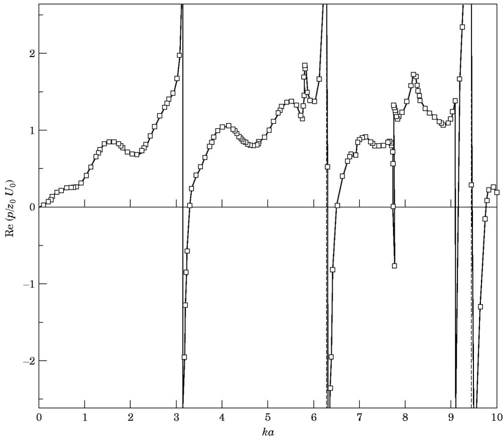
Figure 11. Variation of the real part of the non-dimensional surface pressure at the furthest points of the equatorial circles of two dilating spherical sources, computed by using SHIE, with the non-dimensional wavenumber  $ka$ .
