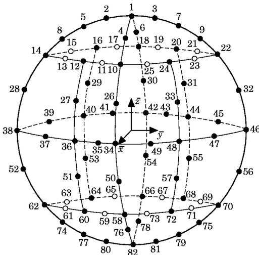
Figure A1. Boundary element discretization of a sphere
