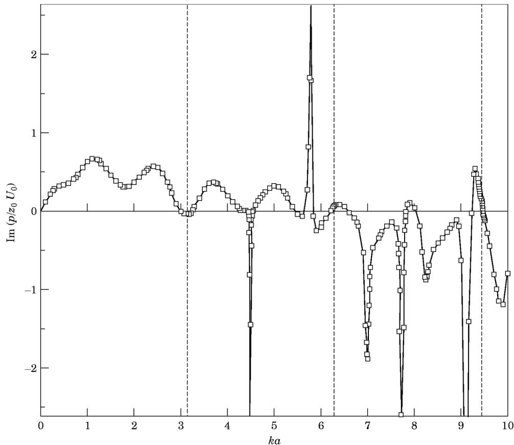
Figure 14. Variation of the imaginary part of the non-dimensional surface pressure at the furthest points of the equatorial circles of two dilating spherical sources, computed by using CHIEF, with the non-dimensional wavenumber  $ka$ .
