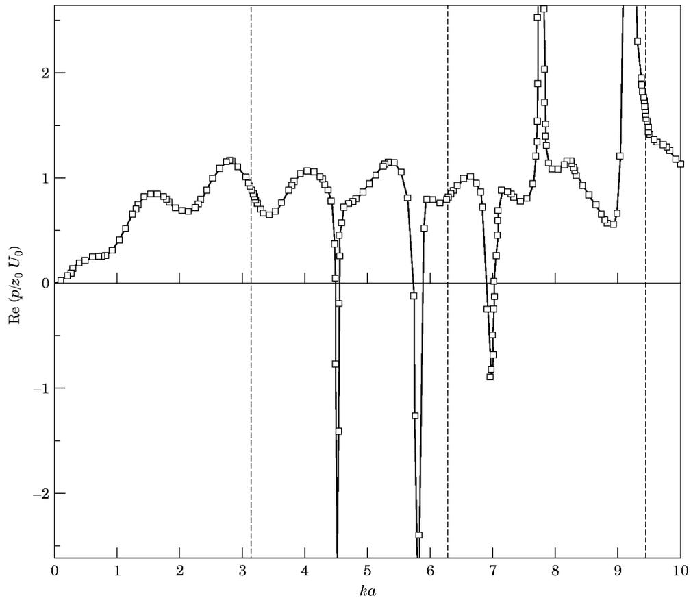
Figure 12. Variation of the real part of the non-dimensional surface pressure at the furthest points of the equatorial circles of two dilating spherical sources, computed by using CHIEF, with the non-dimensional wavenumber  $ka$ .
