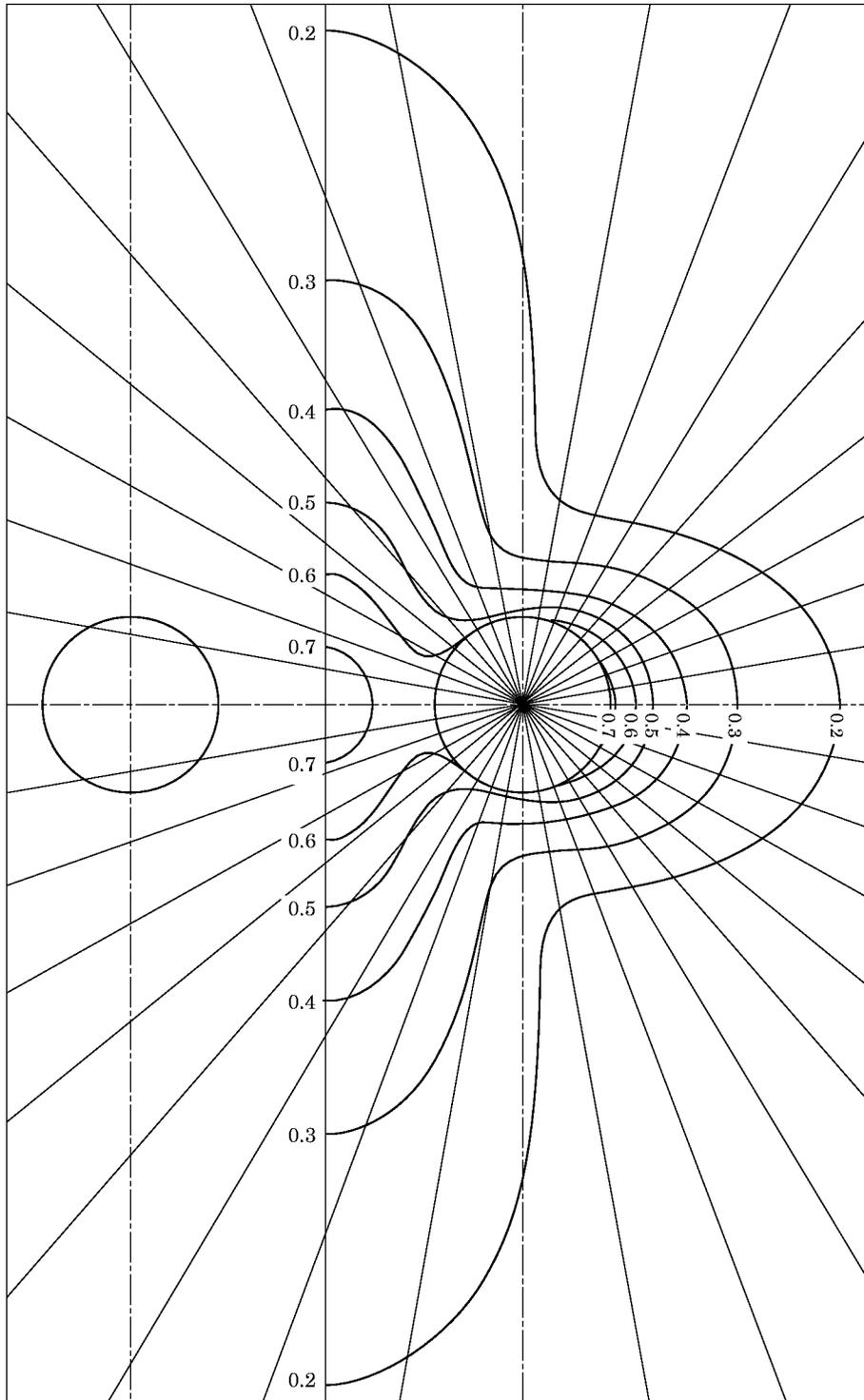
Figure 3. Equal pressure contours of two dilating spherical sources at the  $z = a/3$  plane for  $ka = 1$ .
