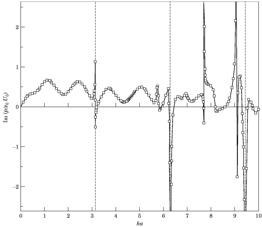
Figure 13. Variation of the imaginary part of the non-dimensional surface pressure at the furthest points of the equatorial circles of two dilating spherical sources, computed by using SHIE, with the non-dimensional wavenumber  $ka$ .
