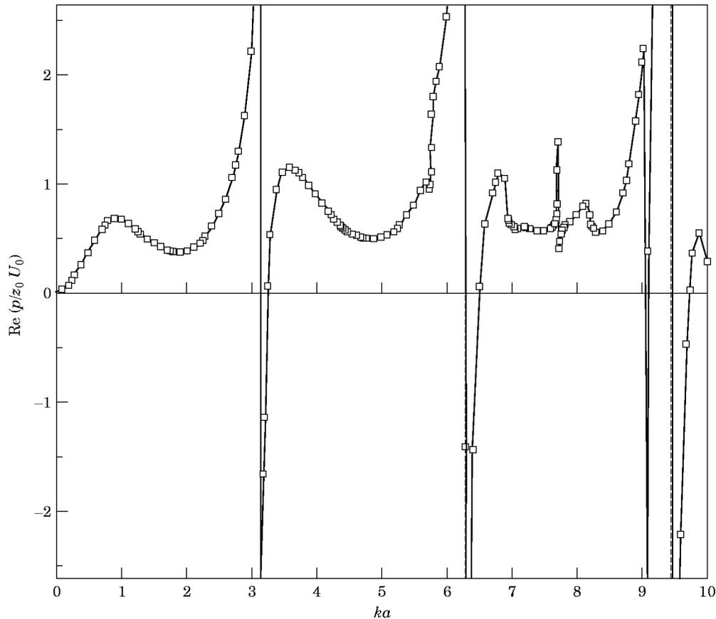
Figure 7. Variation of the real part of the non-dimensional surface pressure at the nearest points of the equatorial circles of two dilating spherical sources, computed by using SHIE, with the non-dimensional wavenumber  $ka$ .
