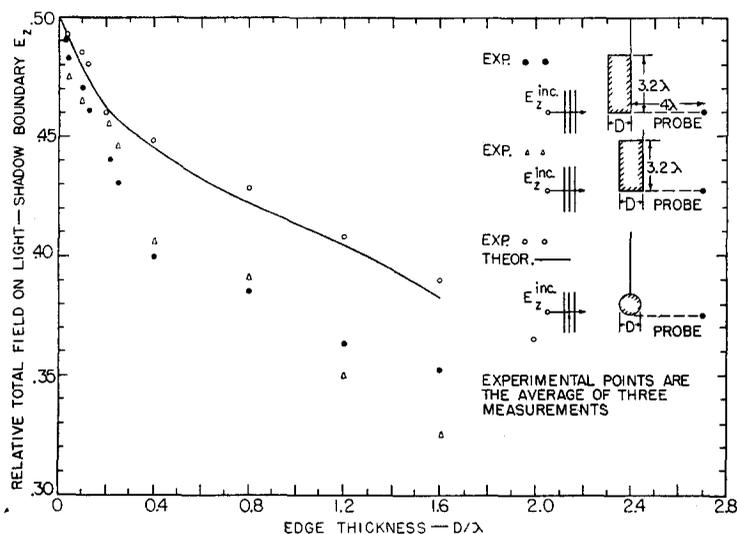
FIG. 11. Measured and theoretical field on the light-shadow boundary for a half plane with a cylindrical edge and measured field for a half plane with a rectangular edge (phase corrected for a line source).
