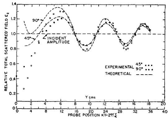
FIG. 6. Approximate theoretical and measured diffraction patterns from 45 and 90 wedges (line source).
