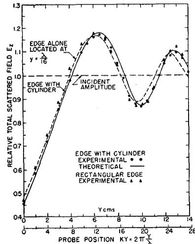
FIG. 10. Theoretical and measured diffraction from a half plane with a circular-cylindrical edge of radius  $=\lambda/16$  and a rectangular edge of thickness  $=\lambda/8$  (line source).
