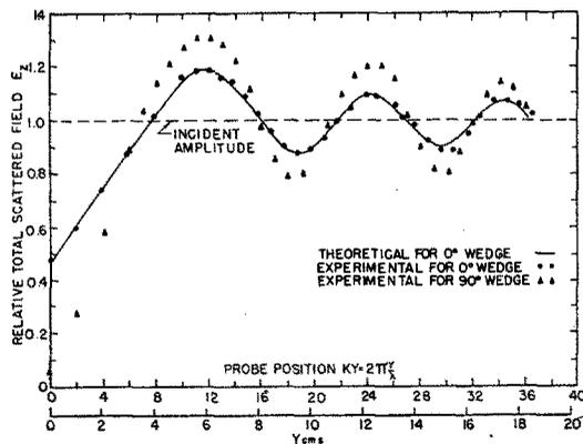
FIG. 5. Measured diffraction patterns from 0° and 90° wedges (line source).
