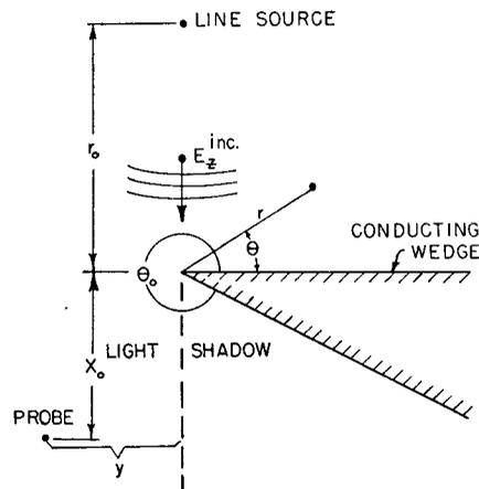
FIG. 3. Coordinate system for scattering from a wedge.
