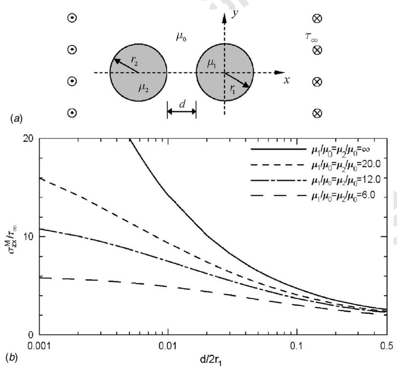
**Fig. 6 (a) Two identical inclusions with centers on the x axis and (b) average shear stress of inclusion versus fiber spacing**
