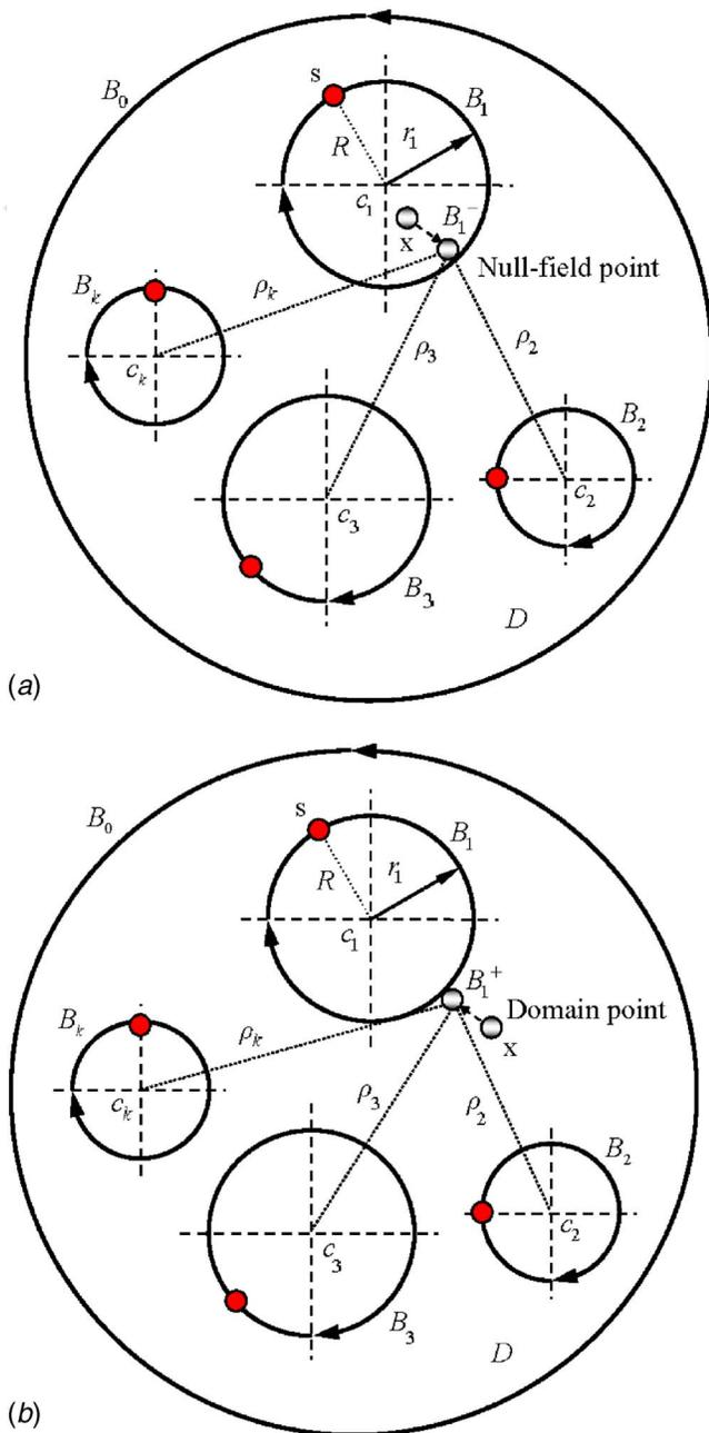
Fig. 3 (a) Sketch of the null-field integral equation for a null-field point in conjunction with the adaptive observer system ( $x \notin D, x \rightarrow B_k$ ) and (b) sketch of the boundary integral equation for a domain point in conjunction with the adaptive observer system ( $x \in D, x \rightarrow B_k$ )
