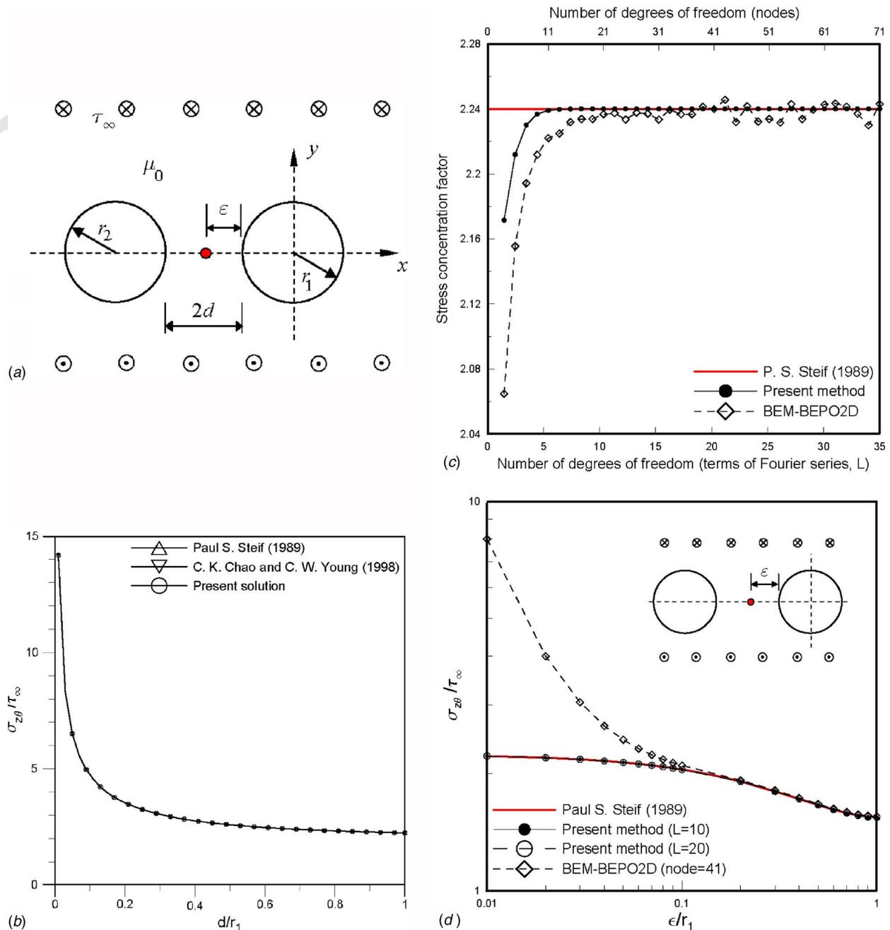
Fig. 5 (a) Two equal-sized holes ( $r_1=r_2$ ) with centers on the  $x$  axis, (b) stress concentration of the problem containing two equal-sized holes, (c) convergence test of the problem containing two equal-sized holes ( $d=1.0$ ), and (d) tangential stress in the matrix near the boundary ( $d=1.0$ )
