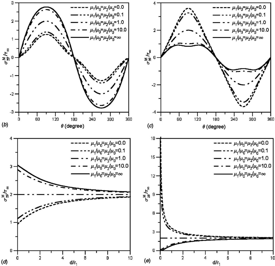
Fig. 10 (a) One hole surrounded by two circular inclusions, (b) tangential stress distribution along the hole boundary with  $\beta=0$  deg, (c) tangential stress distribution along the hole boundary with  $\beta=90$  deg, (d) stress concentration as a function of the spacing  $d/r_1$  with  $\beta=0$  deg, and (e) stress concentration as a function of the spacing  $d/r_1$  with  $\beta=90$  deg
