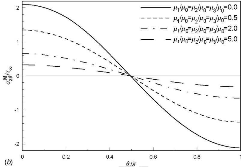
Fig. 11 (a) Three identical inclusions forming an equilateral triangle, and (b) tangential stress distribution around the inclusion located at the origin
