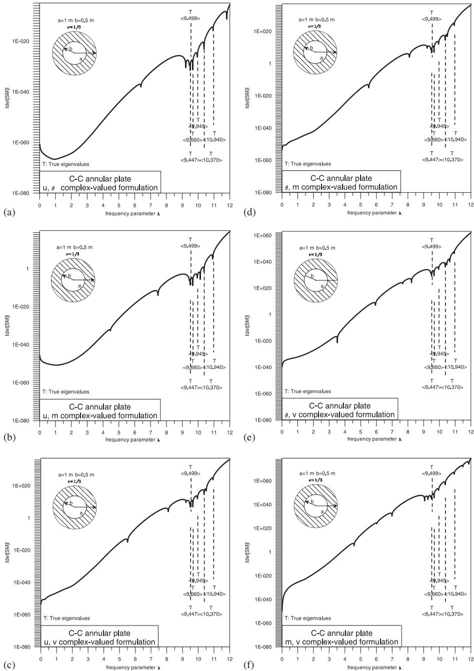
Figure 1. The determinant of the  $[SM^{CC}]$  versus the frequency parameter  $\lambda$  for the C-C annular plate using the six complex-valued formulations.
