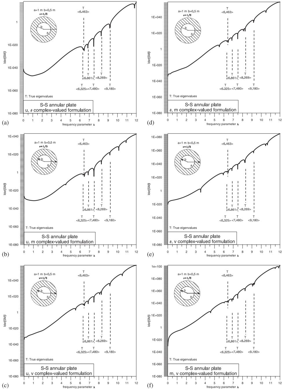
Figure 2. The determinant of the  $[SM^{SS}]$  versus the frequency parameter  $\lambda$  for the S-S annular plate using the six complex-valued formulations.
