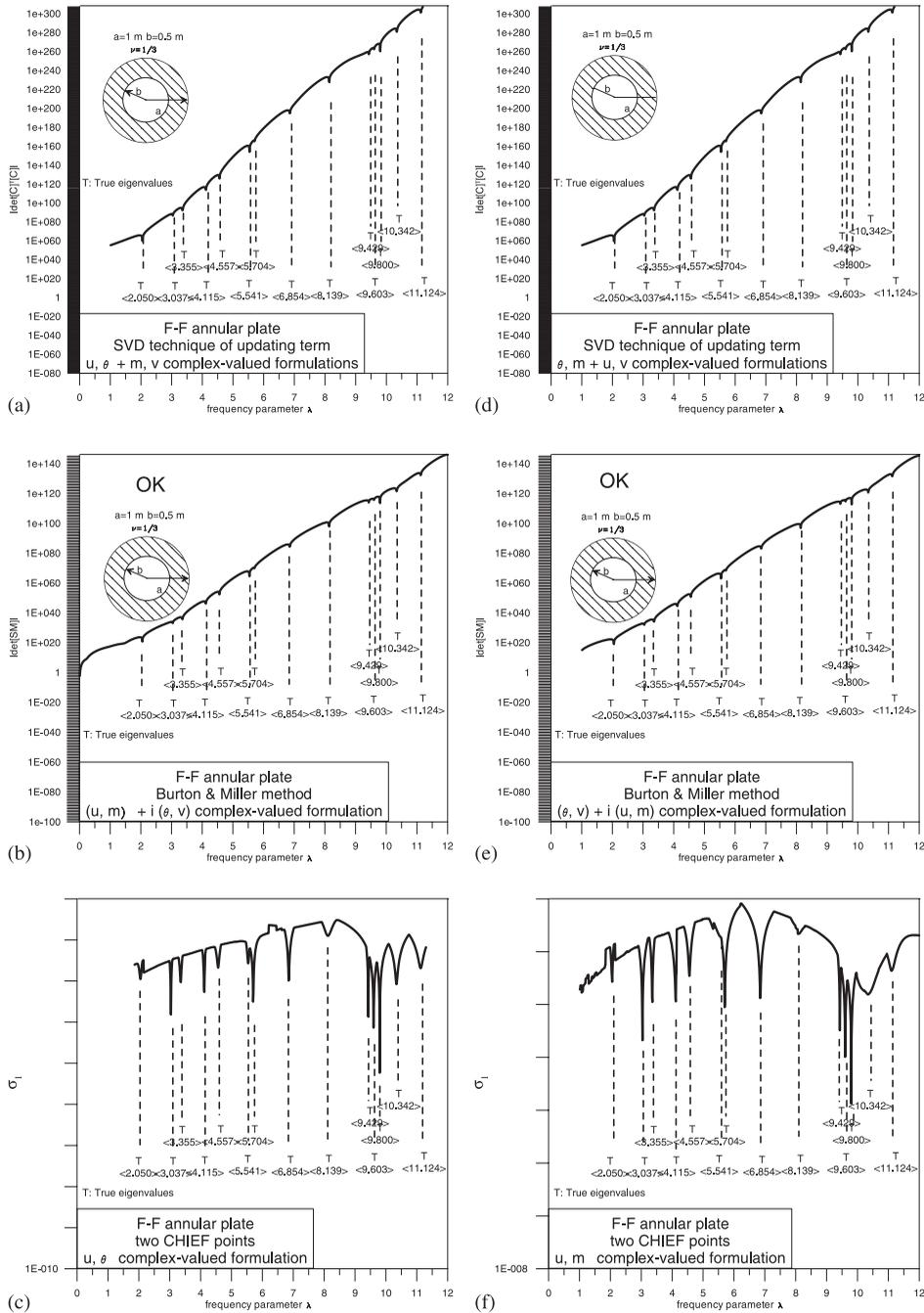
Figure 6. Three alternatives (SVD updating term, the Burton and Miller method and CHIEF method) for the F-F annular plate using the complex-valued formulations.
