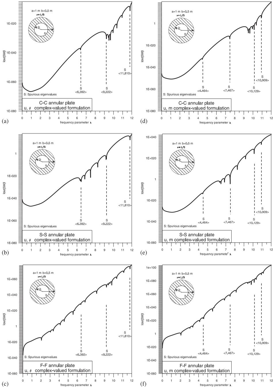
Figure 4. The determinant of the  $[SM]$  versus the frequency parameter  $\lambda$  using the complex-valued formulation ( $u, \theta$  or  $u, m$  formulation) to solve plates subject to different boundary conditions.
