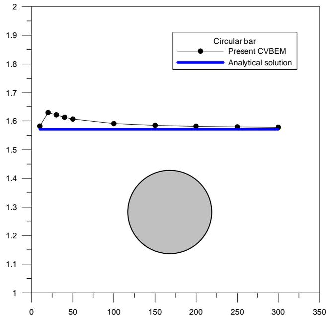
Figure 1. Torsional rigidity versus the number of elements in circular case
