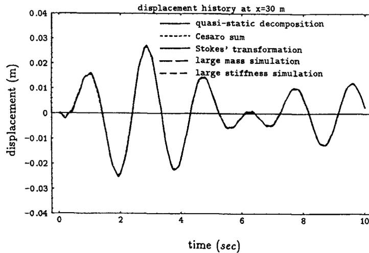
Figure 5. The solutions of in-phase motions at  $x = 30$  using methods (1)–(5) with five modes and 25 elements
