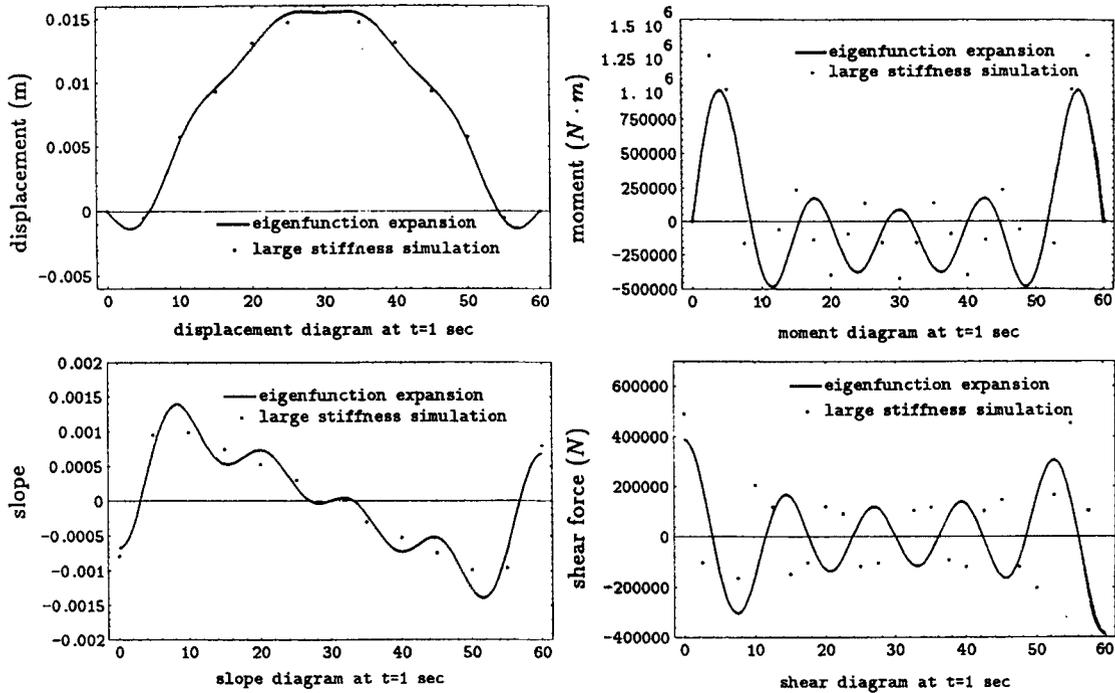
Figure 11. The series solutions for the displacement, slope, moment and shear force at  $t = 1$  s using the eigenfunction expansion method and large stiffness simulation without considering the two largest modes using 10 modes for case 3
