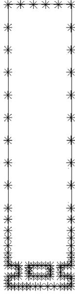
Fig. 4. The related DBEM coarse mesh discretization.
