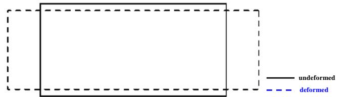
Fig. 4(a) Deformation of an infinite plate subject to a uniform tension
