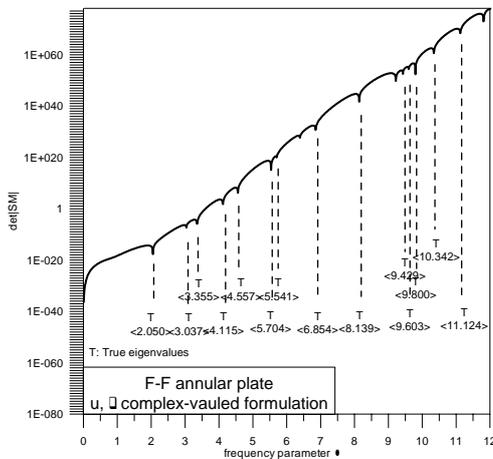
Figure 1.(c)  $Det[SM^{FF}]$  v.s.  $\lambda$  (F-F annular plate)
