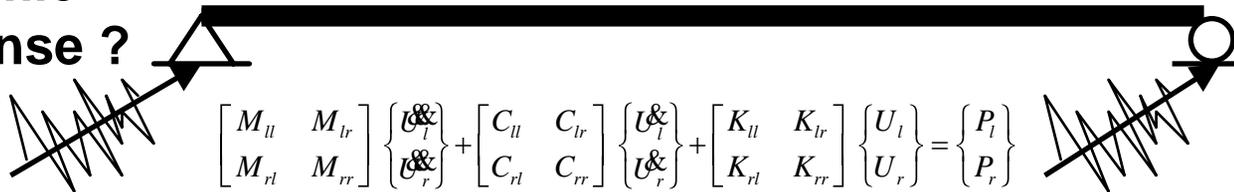
$$\begin{bmatrix} M_{ll} & M_{lr} \\ M_{rl} & M_{rr} \end{bmatrix} \begin{Bmatrix} \ddot{U}_l \\ \ddot{U}_r \end{Bmatrix} + \begin{bmatrix} C_{ll} & C_{lr} \\ C_{rl} & C_{rr} \end{bmatrix} \begin{Bmatrix} \dot{U}_l \\ \dot{U}_r \end{Bmatrix} + \begin{bmatrix} K_{ll} & K_{lr} \\ K_{rl} & K_{rr} \end{bmatrix} \begin{Bmatrix} U_l \\ U_r \end{Bmatrix} = \begin{Bmatrix} P_l \\ P_r \end{Bmatrix}$$
