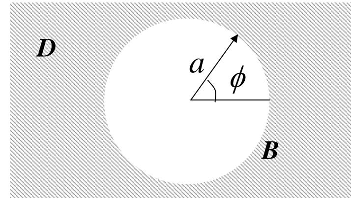
$$\text{Boundary Condition: } u(a, \phi) = \bar{a}_0 + \sum_{n=1}^N \bar{a}_n \cos(n\phi) + \sum_{n=1}^N \bar{b}_n \sin(n\phi)$$
