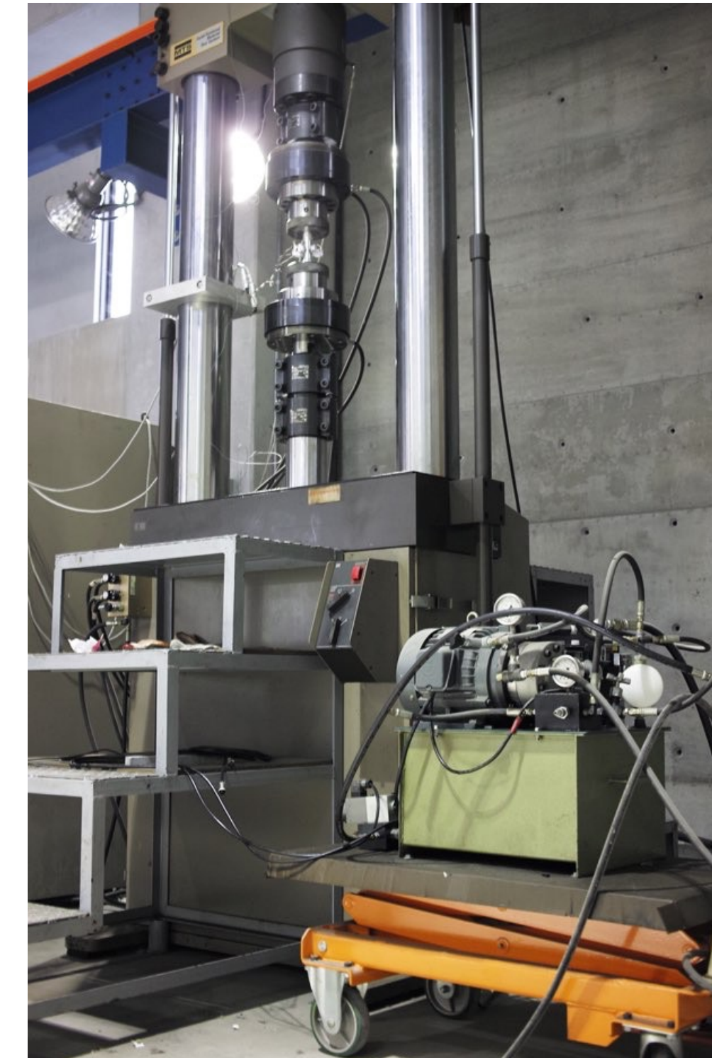
self-made hydraulic system internal pressure: max 68.65 MPa
