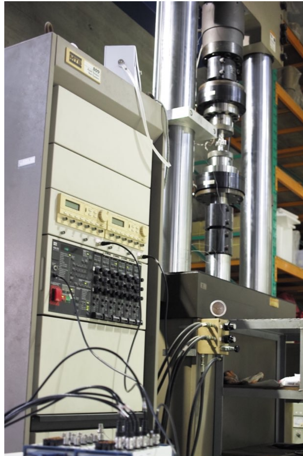
MTS system axial load: max \pm 500 kN torque: max \pm 5500 N-m
